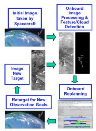
Just as changing cloud patterns on Earth were identified using Earth Observing-1's Advanced Land Imager along with ScienceCraft software, the THEMIS instrument with ScienceCraft on the Mars Odyssey spacecraft can avoid transmitting useless images.
