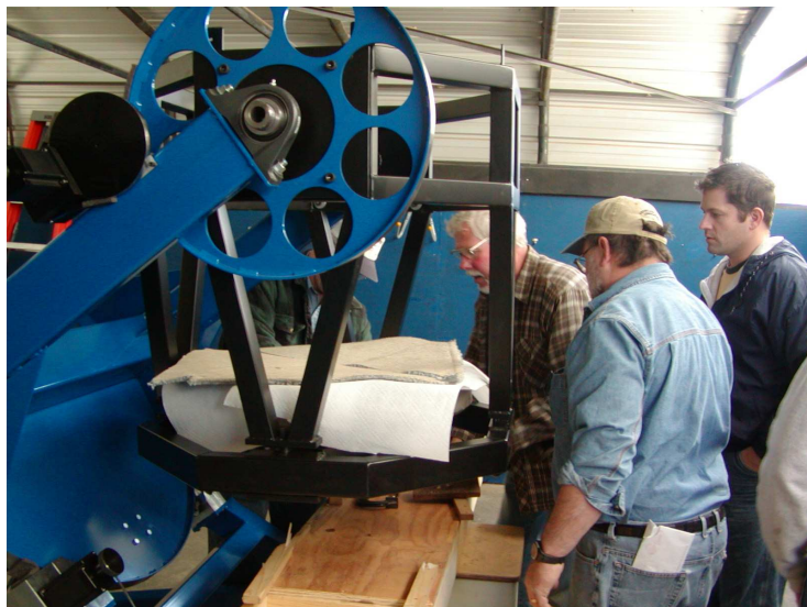
The mirror is protected while mounting mirror cell to scope.
