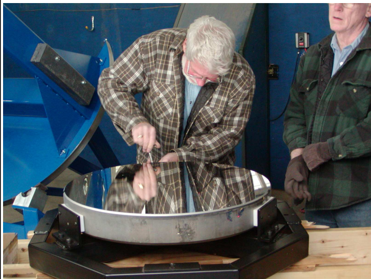
Jerry Foote (ScopeCraft) anchoring the mirror to the cell.
